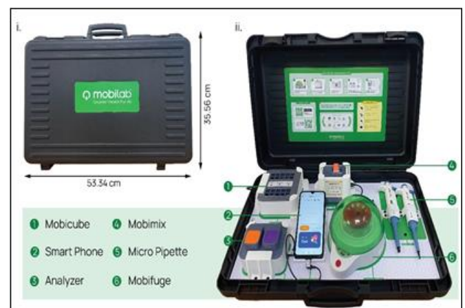
Figure 1: (i) Closed view of Mobilab with a length of 53.34 cm and height of 35.56 cm. (ii) Opened view of Mobilab consisting of (1) Mobicube, a portable battery-operated external incubator that regulates temperature to incubate
