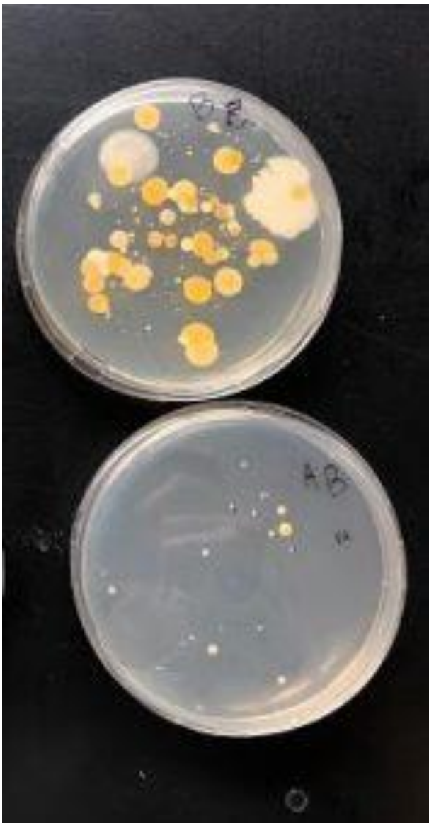
Figure 3 (b): From top to bottom: bacteria before hands were washed with biosand filtered water, bacteria after hands were washed with biosand filtered water
