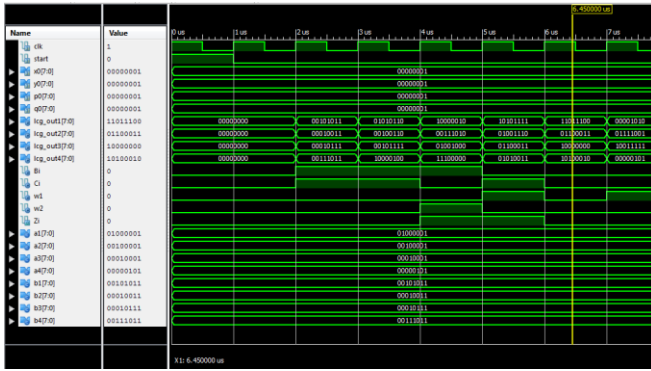
Figure 8: Simulated wave form of Modified Dual CLCG
